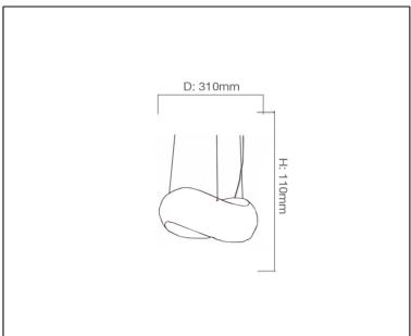
10277 Pendant Light Lamp Type: 1 x T5 Rated input power: 22W
