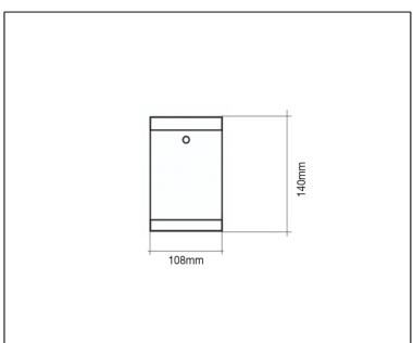
11193 E27 x PAR30 Rated input power: 75W Max Input Voltage: 220-240V
