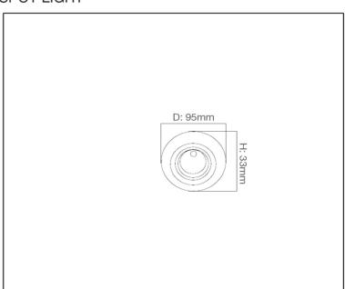
11750 Recessed Fitting Lamp Type: G5.3 MR16 Wattage: 50W
