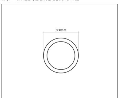
11787 LED with built-in motion sensor Rated input power: 16W Input Voltage: 220-240V
