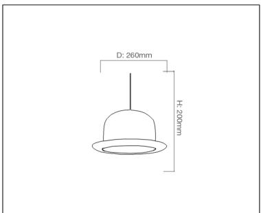
11865 Pendant Light Lamp Type: E27 Rated input power: 60W
