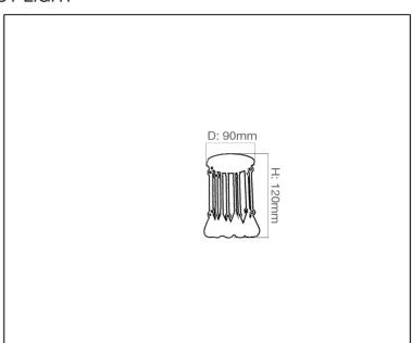
12906 Recessed Fitting Lamp Type: MR 16/LED Wattage: 50W
