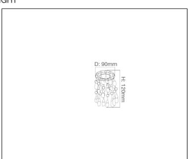
12908 Recessed Fitting Lamp Type: MR 16/LED Wattage: 50W
