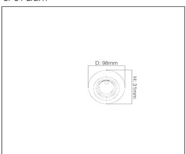
13493 Ceiling Mounted Lamp Type: MR 16/COB LED Wattage: 50W
