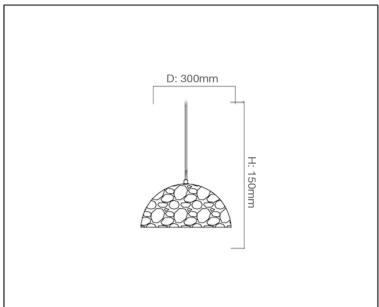
13986 Pendant Light Lamp Type: E27 Rated input power: 60W
