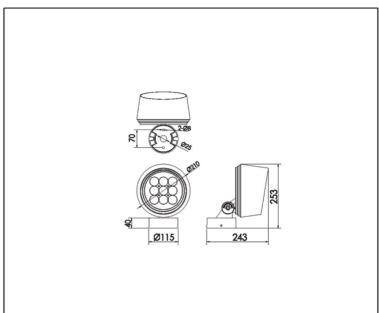
14121 CREE LED Rated Luminaire Luminous Flux: 4275lm Rated input power: 45W Luminaire Efficiency: 95lm/W Input Voltage: AV90-265V
