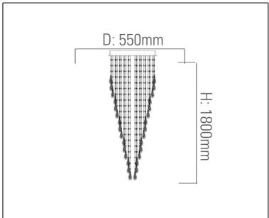
14345 Suspended Mounted Lamp Type: GU10 x 7 Rated input power: 40W Max
