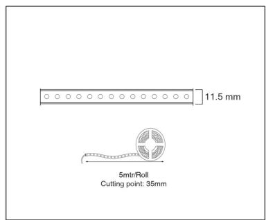
14500 CREE LED Rated Luminaire Luminious Flux: 840lm/M Rated input power: 13W/Meter
