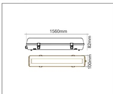
14725 LG LED Driver: Tridonic Rated Luminaire Luminous Flux: 6750lm Rated input power: 54W Luminaire Efficiency: 125lm/W Input Voltage: 220-240V
