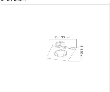
13495 Recessed Fitting Lamp Type: MR 16/COB LED Wattage: 50W
