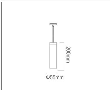
14942 CREE LED Rated Luminaire luminous flux: 360lm Rated input power: 7W Luminaire efficiency: 51lm/W Input voltage: 220-240V
