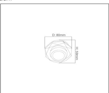
10738 Recessed Fitting Lamp Type: 3 x Cree LED Wattage: 1W
