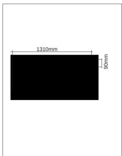
11333 T5 Light source Rated input power: 2 x 28W Input voltage: 220V
